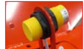
Fill Level Sensor Signals when hopper is low on seed.
