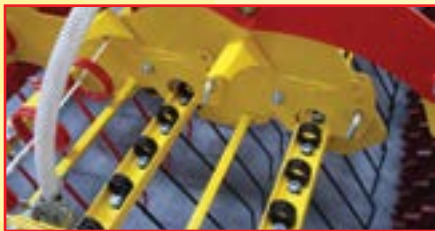
Adjustable 0.3" tines allow for more or less aggressive field operation.
