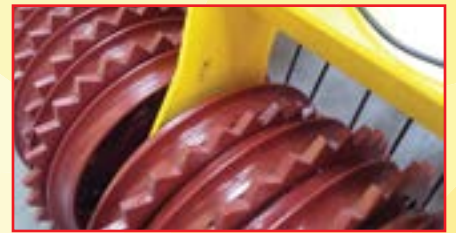
Cambridge roller for existing grass operations.
