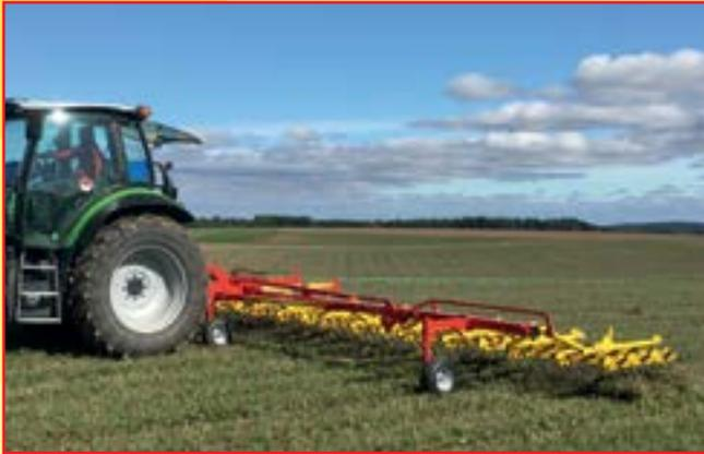
The AS Series Tined Weeders efficiently pull out weeds that have germinated, leaving them on the soil surface to wither. Approximately 90% of germinated weeds are stopped in their tracks. With the available widths of 19.8 ft, 29.6 ft, and 39.4 ft for the AS 600 M1, AS 900 M1, and AS 1200 M1, respectively, there is a tined weeder for every operation. Plus, these weeders are great combined with our PS 300 – PS 500 Air Seeders. Great for organic operations.
